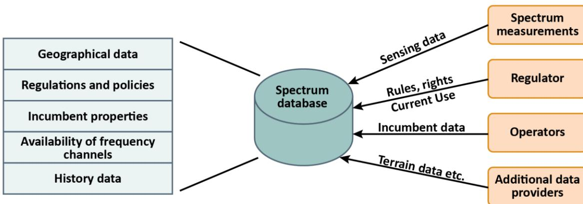
*Figure 4- A general spectrum database model. (Source: M. Höyhtyä, et al.)<sup>15</sup>*
