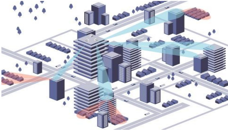
Figure 24: Fixed wireless access using database-enabled frequency reuse in millimeter bands
