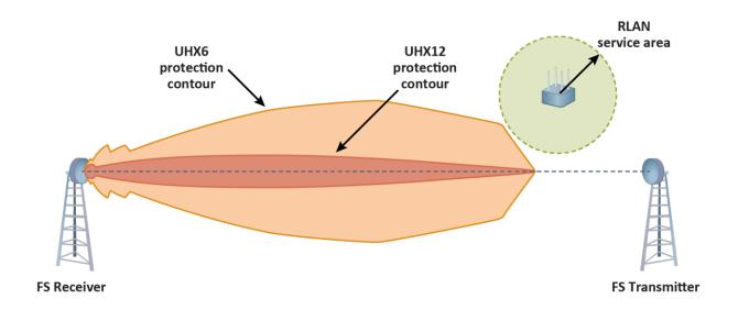
Figure 20: The AFC system enforces 3D Protection contours to avoid RLAN interference to Fixed Service receivers.<sup>110</sup>
