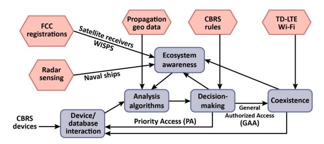
Figure 14: Admission control system architecture for three-tier, FCC-certified Spectrum Access System.
