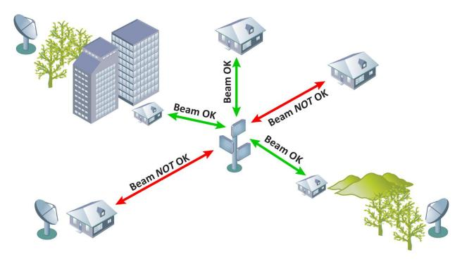
Figure 22: Automated frequency coordination of directional PtP fixed wireless with FSS earth stations. Unlike mobile use, fixed PtMP is inherently directional and can be sectorized to coexist with FSS.
