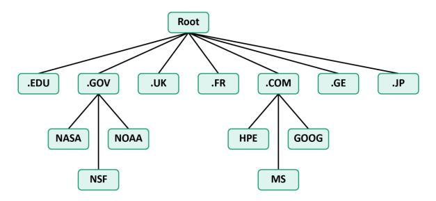
Figure 3: The Internet's Domain Name Service (DNS) is a distributed database process that connects domain names to IP addresses to facilitate the routing of Internet traffic.<sup>13</sup>
