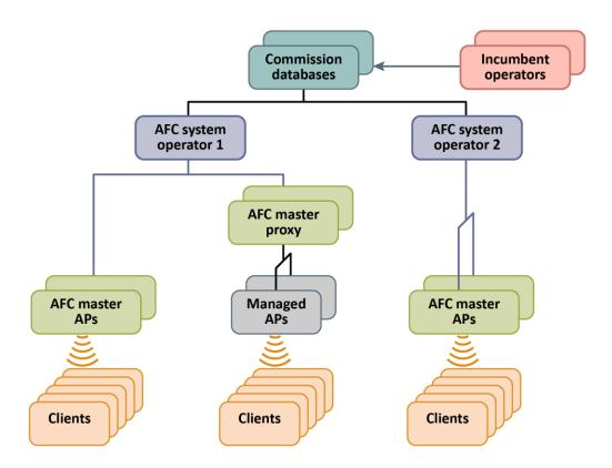
Figure 19: Simplified architecture for Automated Frequency Coordination in 6 GHz band.
