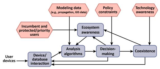
Figure 5: Conceptual architecture for an automated frequency coordination (AFC) system.
